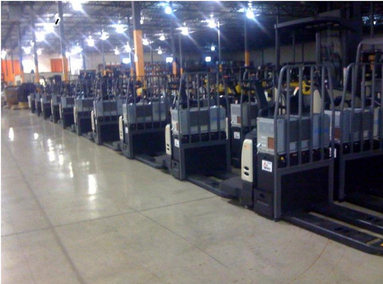
**Figure 2. Class III forklifts with Oorja products serving as battery range extenders**
