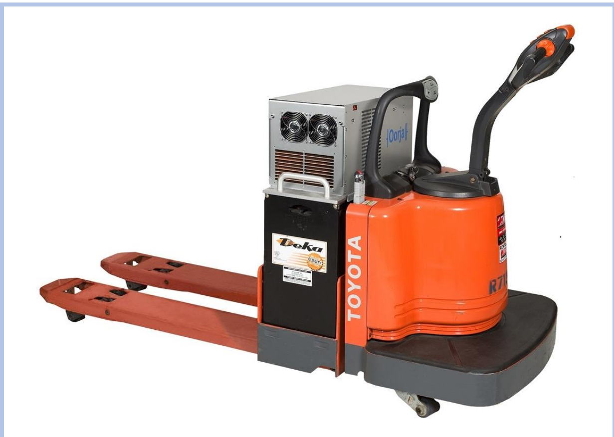
Figure 1. An Oorja Model 3 on a Class III forklift
