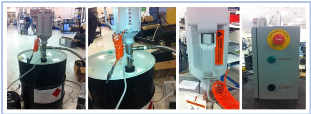
Figure 1. The Oorja Mobile Refueling Station, showing (from left to right) the pump inserted into a 55-gallon drum, the pump connections, a close-up of the pump, and the electrical box that shows the Start button, the green light that shows when pumping is active, and the emergency Stop button.
